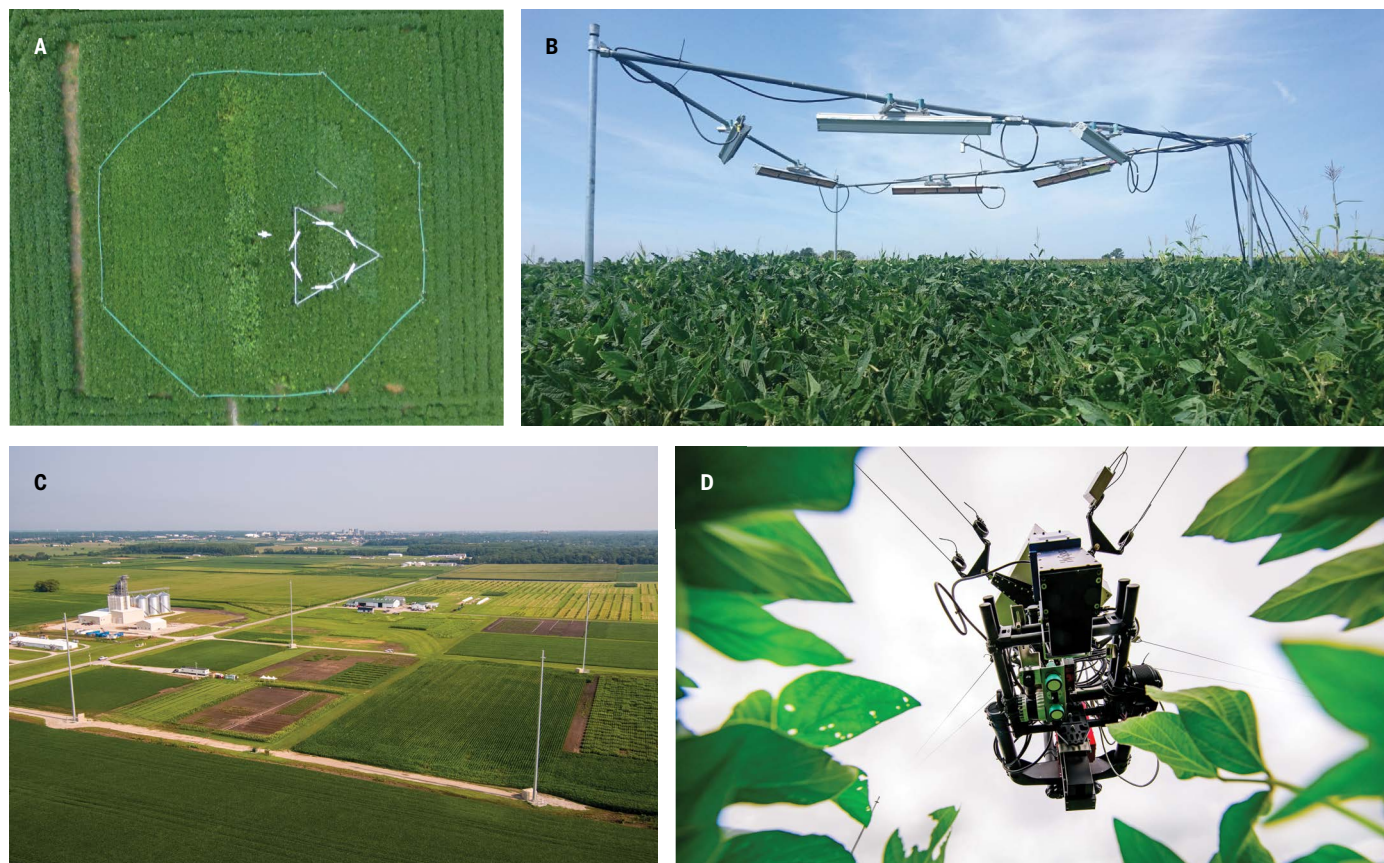
Fig. 3. Experimental techniques for understanding high-temperature impacts and tolerance in crop germplasm in farm fields. Aerial view within an elevated CO 2 plot (A) and lateral view (B) of an in-field infrared heating array used to simulate warmer growing conditions for crops at the Soybean Free Air Concentration Enrichment facility (SoyFACE) in Urbana, Illinois. The electrical current to six infrared heaters is modulated to maintain a set point canopy temperature above a nonheated reference area adjacent to the heated area, as determined from thermal imaging of the canopy. As temperatures fluctuate over the reference plot, output from the heaters is adjusted to match the target temperature increase for the heated plots. Various experiments have been undertaken to simulate global warming (80) and heat waves (81) and to test strategies to genetically improve crop resilience to temperatures (63, 66). (C) Aerial view of the 4-Ha RIPE Aerial Plant Phenotyping System (RAPPS) located on the Energy Farm of the University of Illinois Urbana-Champaign and (D) a view of the sensor package, including hyperspectral imagers, light detecting and ranging (lidar), thermal photography, and RGB photography sensors, mounted on the dolly. RAPPS can move the sensor package over the 4 Ha of farmland to provide ultra-high-resolution, repeatable, semiautonomous, rapid, and high-accuracy information on more than 100,000 individual plants. RAPPS is highly versatile and can provide high-throughput information to advance breeding efforts for improved thermal resilience in crops using natural variation in temperatures or, alternatively, by integrating high-temperature treatments [(A) and (B)] into the measurement footprint.
